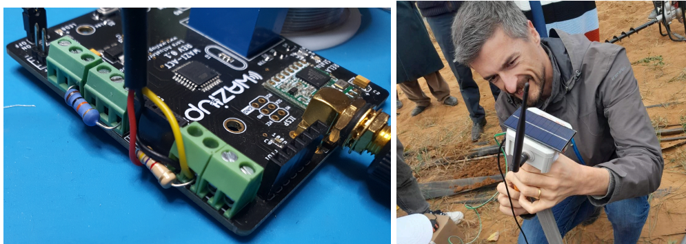
Figure 11: WaziSense microcontroller wired (left), Installation of the Smart Tensiometer (right)
